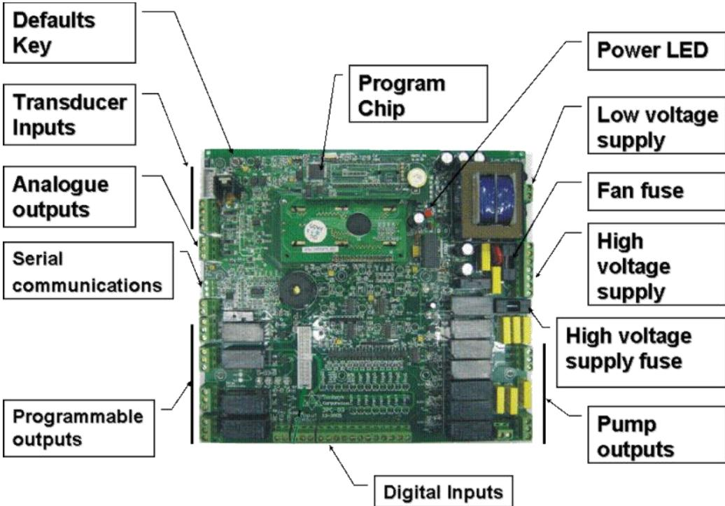
Detailed above are the locations for the components for the Swordfish+ Circuit Board
