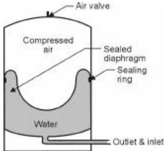
As with all pressure systems a pressure tank is recommended for use in pressure systems. The pressure tank is used to:
