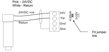
After fitting the transducer, calibration will be required.
