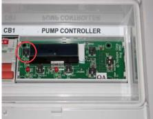
Activating one of the inputs will display an "X" for the applicable input.
