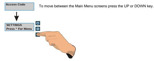
To access a sub menu press the ENTER " \* " key. Access to the sub menus is controlled by an Access Code which can be entered prior to accessing the sub menu or if it has not been entered it will pop up allowing it to be entered prior to accessing any of the sub menu. If the Access Code is not entered correctly the system will disable entry into the Sub menus and the use of any pump select or enable keys.
